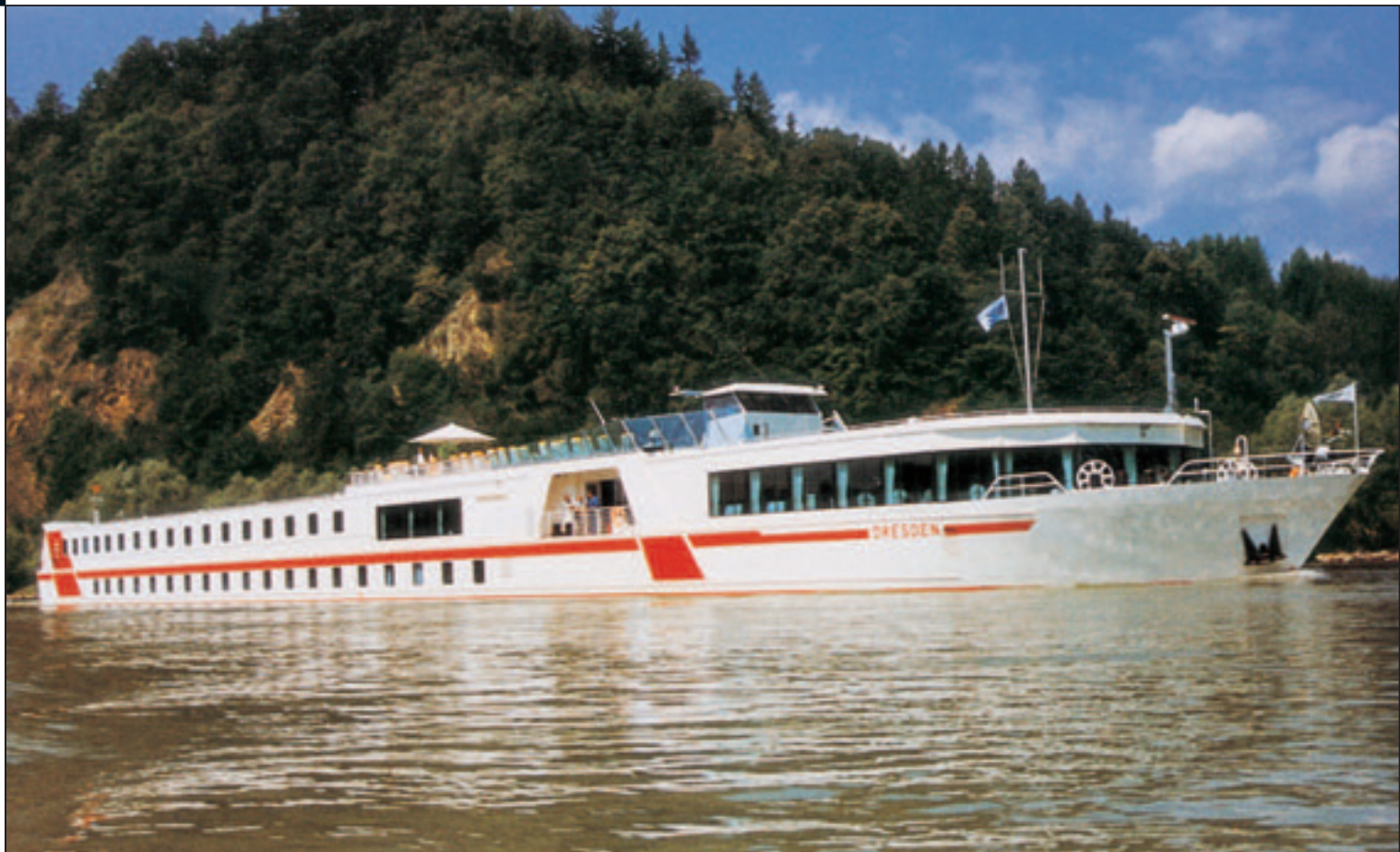
River cruise vessel (0.90 m draught), 3 x SPJ 82 (340 kW each) stern installation, 1 x SPJ 57 (190 kW) bow installation Shipyard: DWE Deggendorfer Werft & Eisenbau GmbH, Germany Owner: Peter Deilmann Reederei GmbH & Co., Germany
