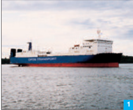
1 Ro-Ro vessel (8.40 m draught), 2 x SPJ 220 (850 kW each) Owner: DFDS AS, Denmark
