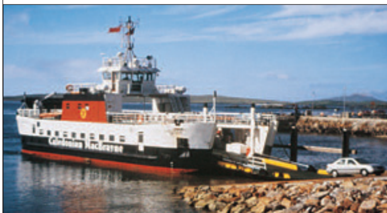
Double-ended ferry (1.40 m draught), 2 x SPJ 132 (505 kW each) Shipyard: McTay Marine Ltd., United Kingdom Owner: Caledonian MacBrayne, United Kingdom
