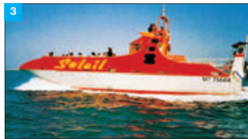
Smaller Standard Vessel (1.64 m draught), 2 x SPJ 82 (370 kW each) Shipyard: Danyard Aalborg AS, Denmark Owner: Royal Danish Navy
