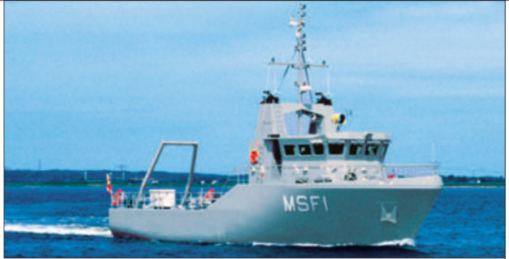
Smaller Standard Vessel (1.64 m draught), 2 x SPJ 82 (370 kW each) Shipyard: Danyard Aalborg AS, Denmark Owner: Royal Danish Navy
