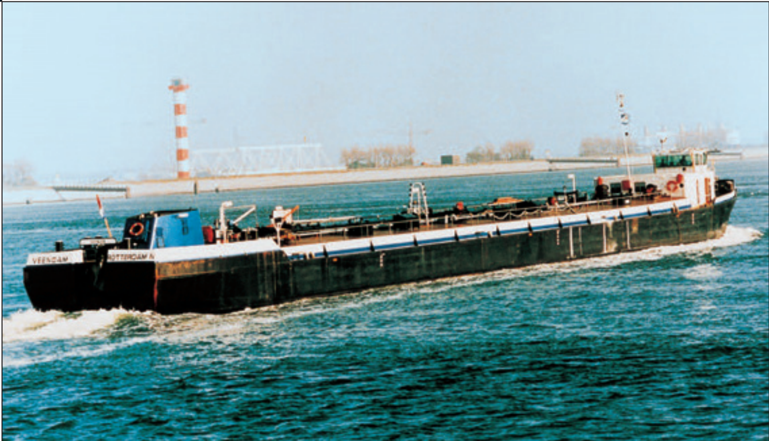
Inland water tanker (2.50 m draught), 2 x SPJ 82 (340 kW each) Conversion yard: Slob & Dolderman, The Netherlands Owner: VTR Verenigde Tankrederij Rotterdam, The Netherlands
