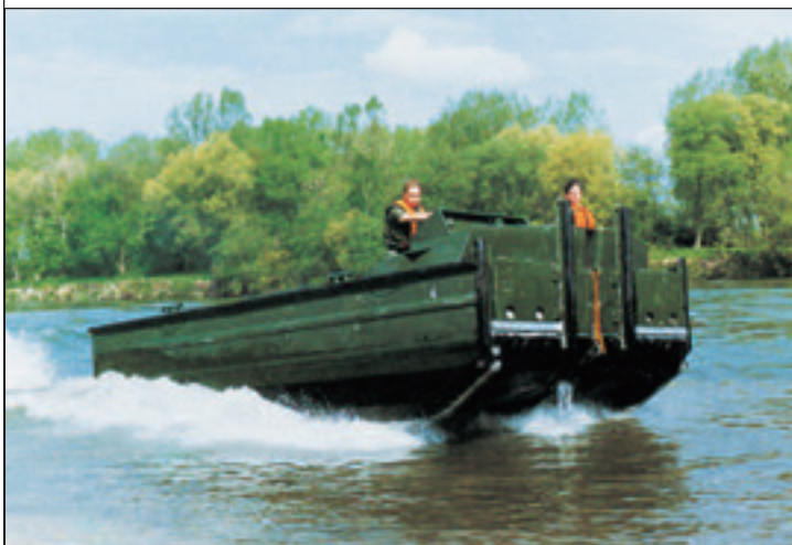
Bridge erection boat (0.45 m draught), 2 x SPJ 55 M (131 kW each) Shipyard: SCHOTTEL GmbH & Co. KG, Germany Owner: German Federal Armed Forces
