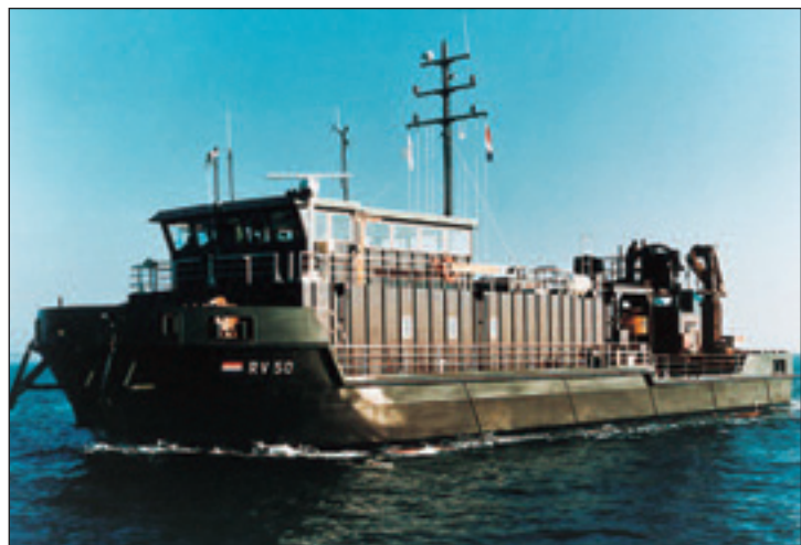
Diving support vessel (1.50 m draught), 1 x SPJ 57 (250 kW) Shipyard: Vervako BV, The Netherlands Owner: Royal Dutch Navy
